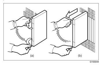
**Note:** The ejectors latch on to a pin on the card. If the ejectors will not open, pinch them to raise them up and off the pin.
