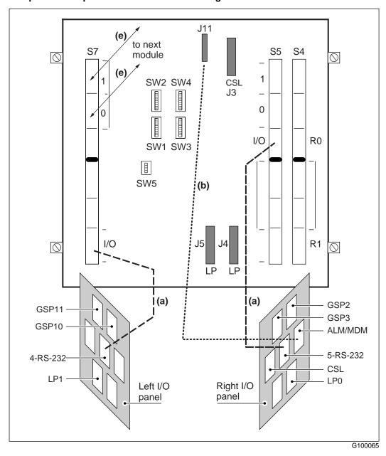
Installing cables from backplane to I/O panel
