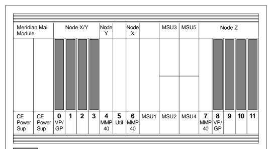
VP card slots. VP8 cards can go in any of the slots numbered 0 to 2 or 8 to 10, while VP4 cards can only go in slots 2 to 3 or 10 to 11, depending on the configuration.
