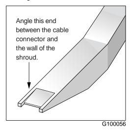
**Note:** If the straight end of the tool is notched, use that end if you can access the connector straight-on. If you must angle the tool at all, use the angled end.
