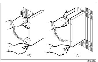
2 Check each card to make sure that there are no loose parts and that the card is not bent.
