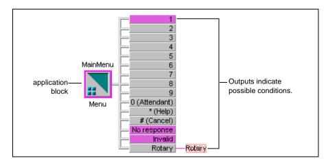
The outputs are the different conditions that can occur. For example, in the Menu block, one of the following conditions may occur:
