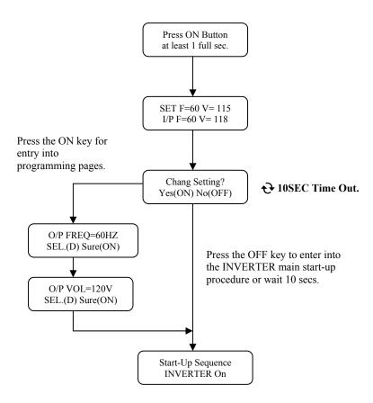
SET = Last Programmed Setting for Operation I/P = Bypass Circuit Sensor – If Present.
