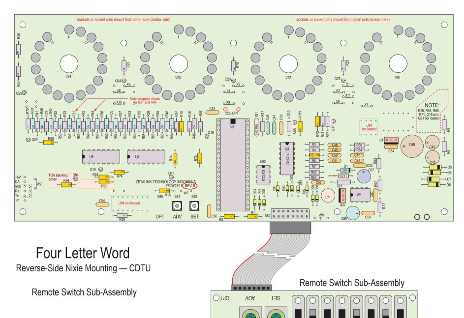
Header mounted on reverse side from switches
