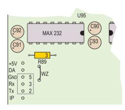
Serial RS-232 Input Option detail of affected components only Components supplied by user.
