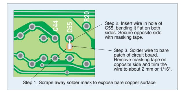
The view shown is from the component side. C55 is located near U3. The repair shown above may have already been performed on the board shipped in your kit, since it can be quite easy for an experienced person yet remain difficult for inexperienced hands. Two photographs of completed repair work along with more detailed instructions can be found on this Zetalink web page: <<u>http://zetalink.biz/FLGKerrfix.html></u>
