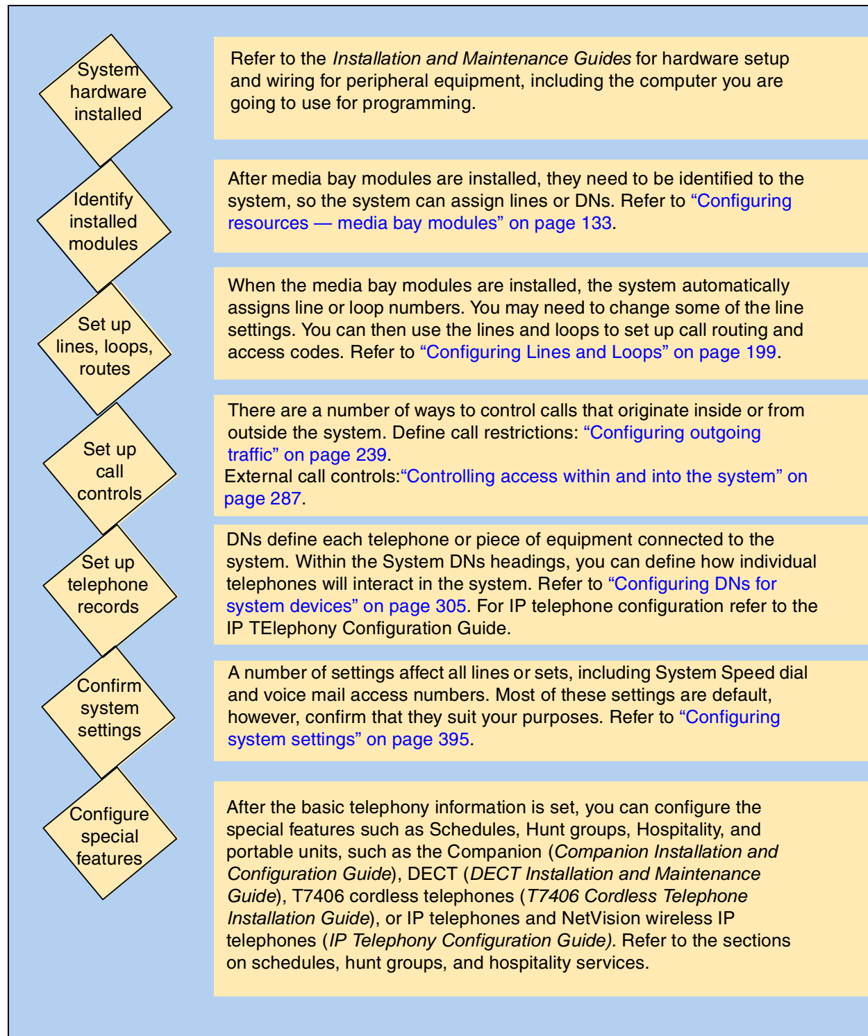
Figure 45 Tasks for installing the telephony components
