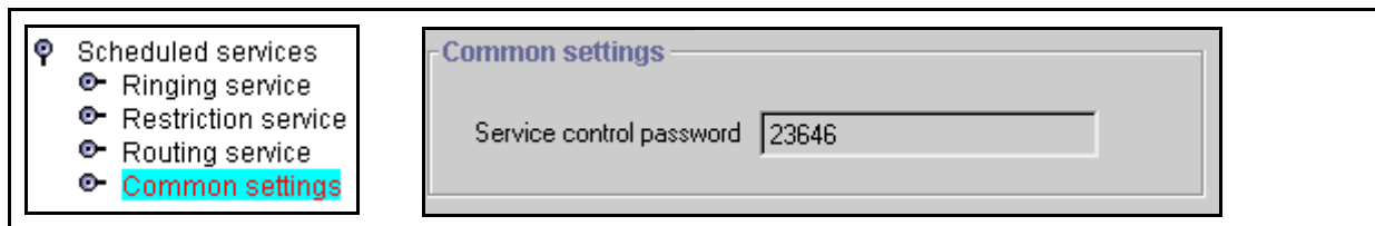
Figure 147 Entering the Service control password
